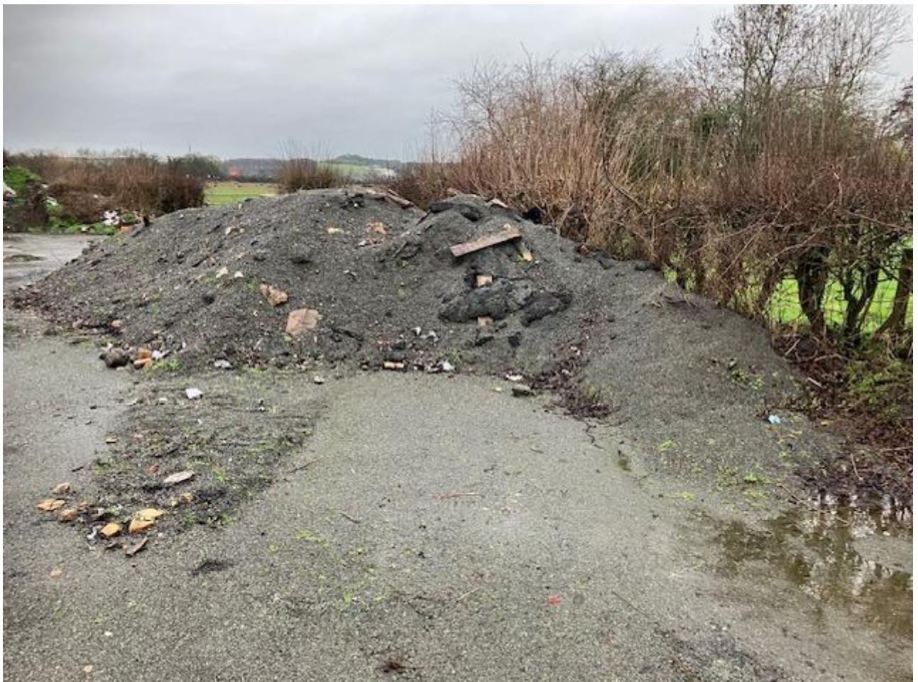
Used road plainings in the layby
