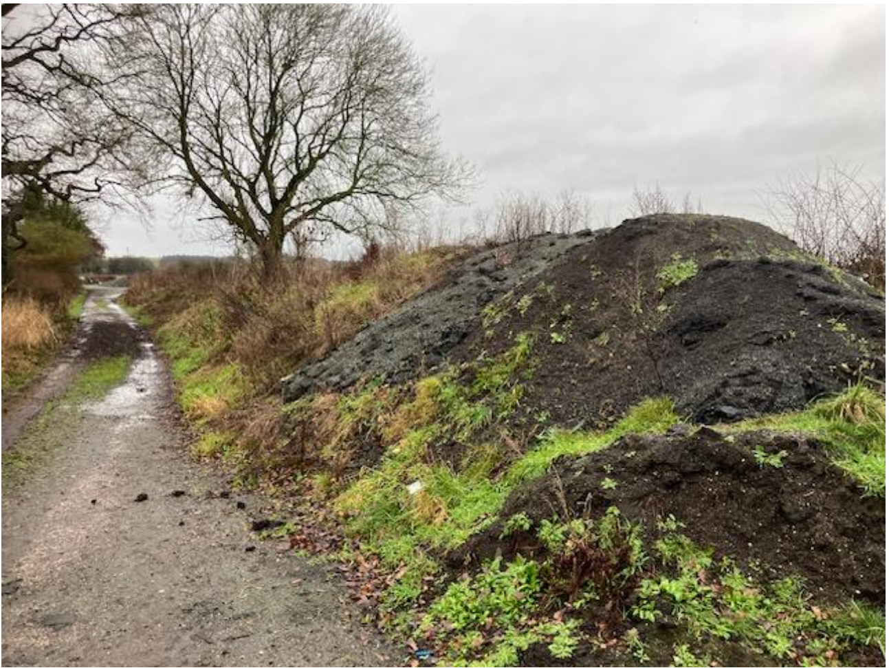
Used road plainings in the layby
